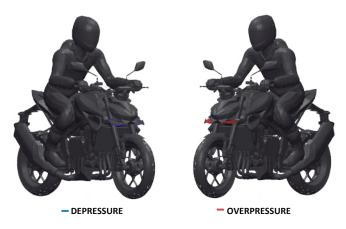
Due to its angles and frontal surface, it creates an overpressure on the top of the spoiler. The turbulance create below, generates a difference of pressure between the upper and lower part of the spoiler. Which ultimately generates the aerodynamic downforce.
