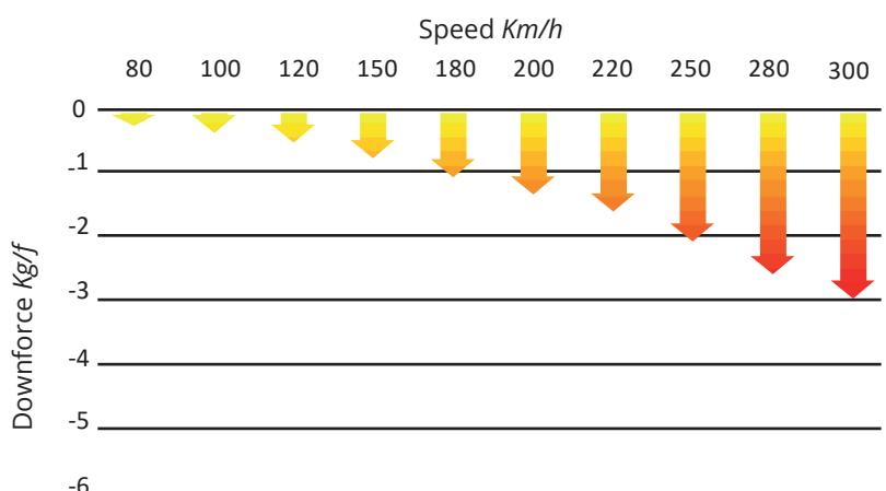
The Downforce that the spoilers generates raises potentially as the speed increases, at top speed we get 2,5 Kg/f.
