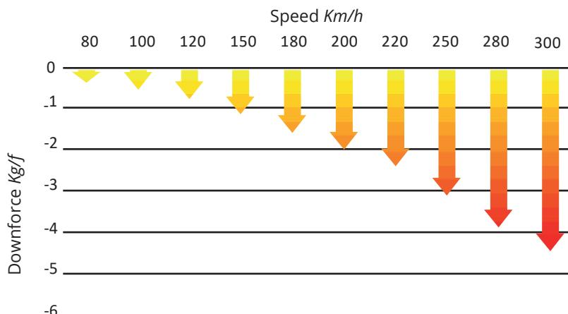
The Downforce that the spoilers generates raises potentially as the speed increases, at top speed we get 2 Kg/f.
