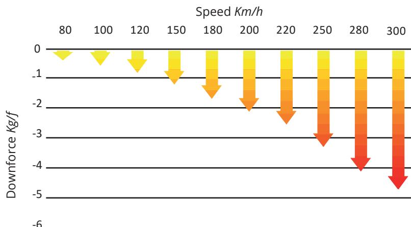
The Downforce that the spoilers generates raises potentially as the speed increases, at top speed we get 3,3 Kg/f.
