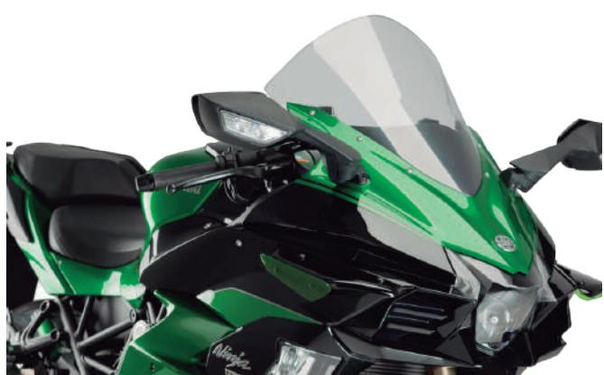
The Downforce that the spoilers generates raises potentially as the speed increases, at 200 km/h we get 1,8 Kg/f.
